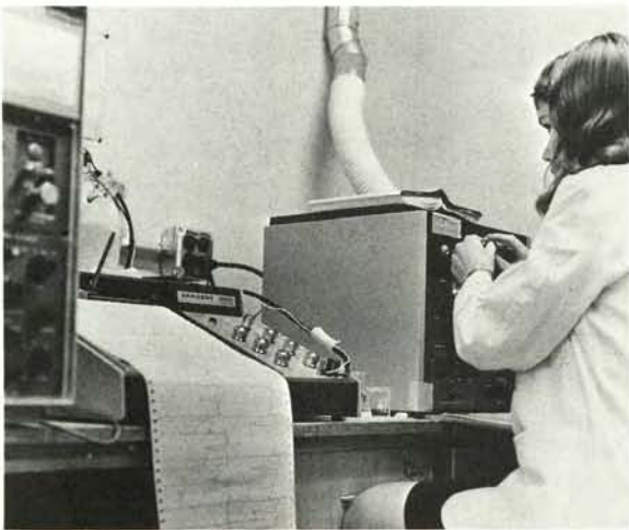
A research assistant injects pesticide samples into a gas chromatograph.
