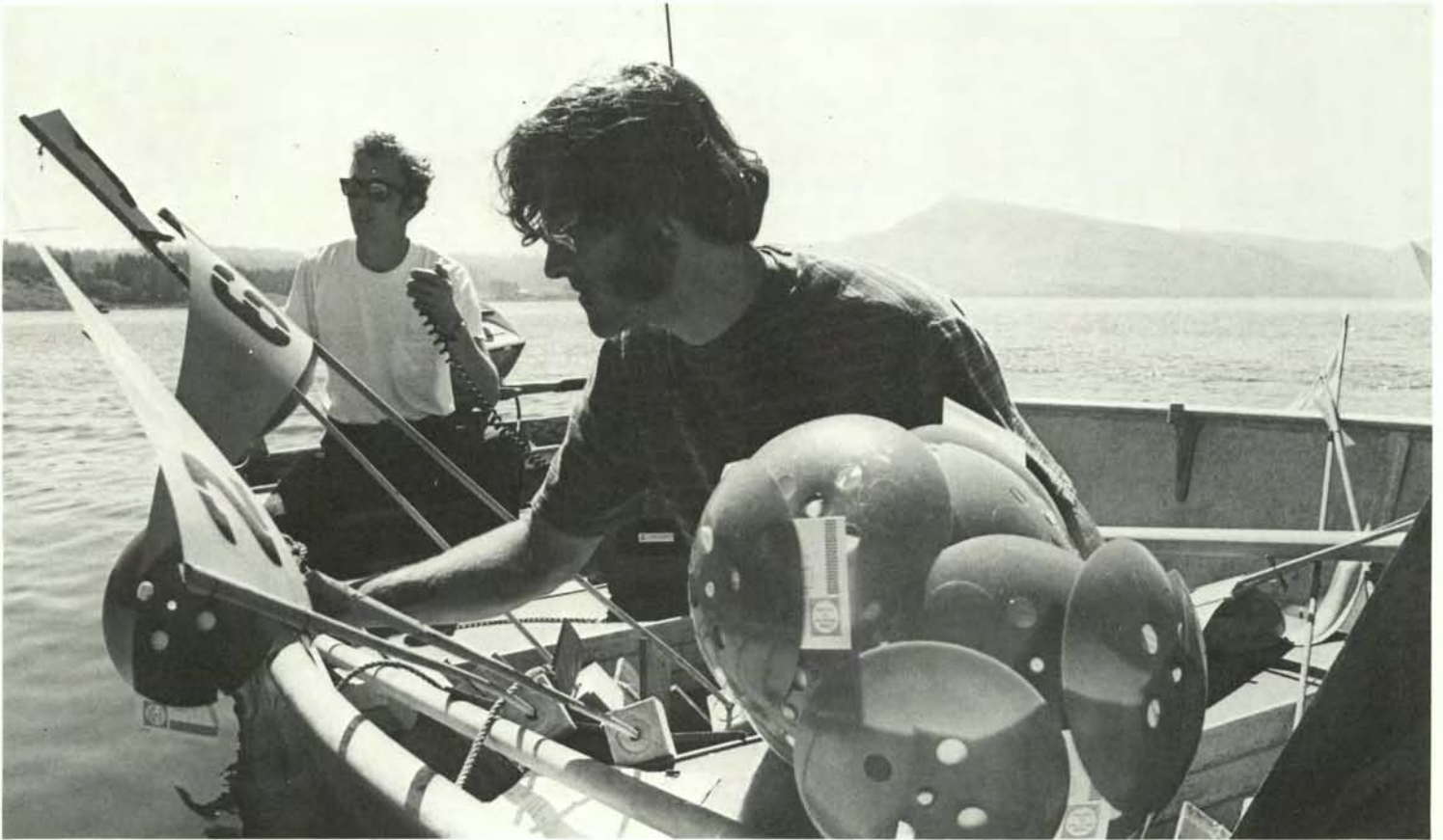
OSU ocean engineers Scott Boley, left, and Bill Mullenhoff place disc shaped bottom drifters in a bay. These drifters are used for gathering engineering data for future Oregon planning.
