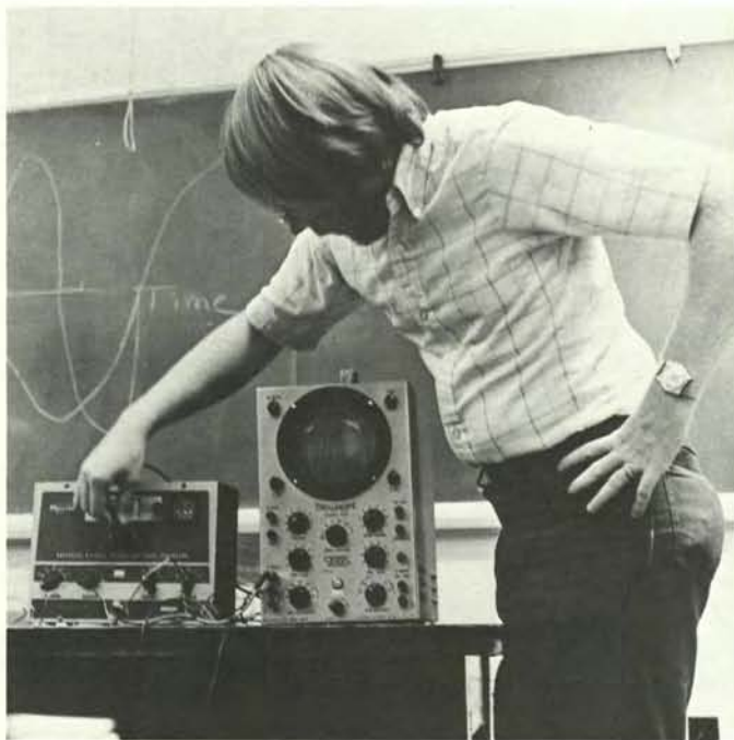
Joseph Joncus explains a pulse generator and oscilloscope to a ham radio class.
