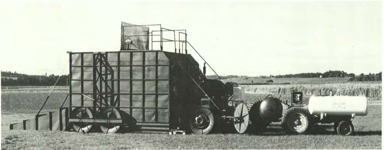
Straw field sanitizer burns straw with minimum of air pollution.
