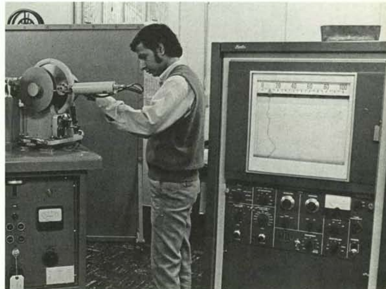
This x-ray metallography process bombards a crystalline structure with x-rays to determine many of the crystal's important properties.
