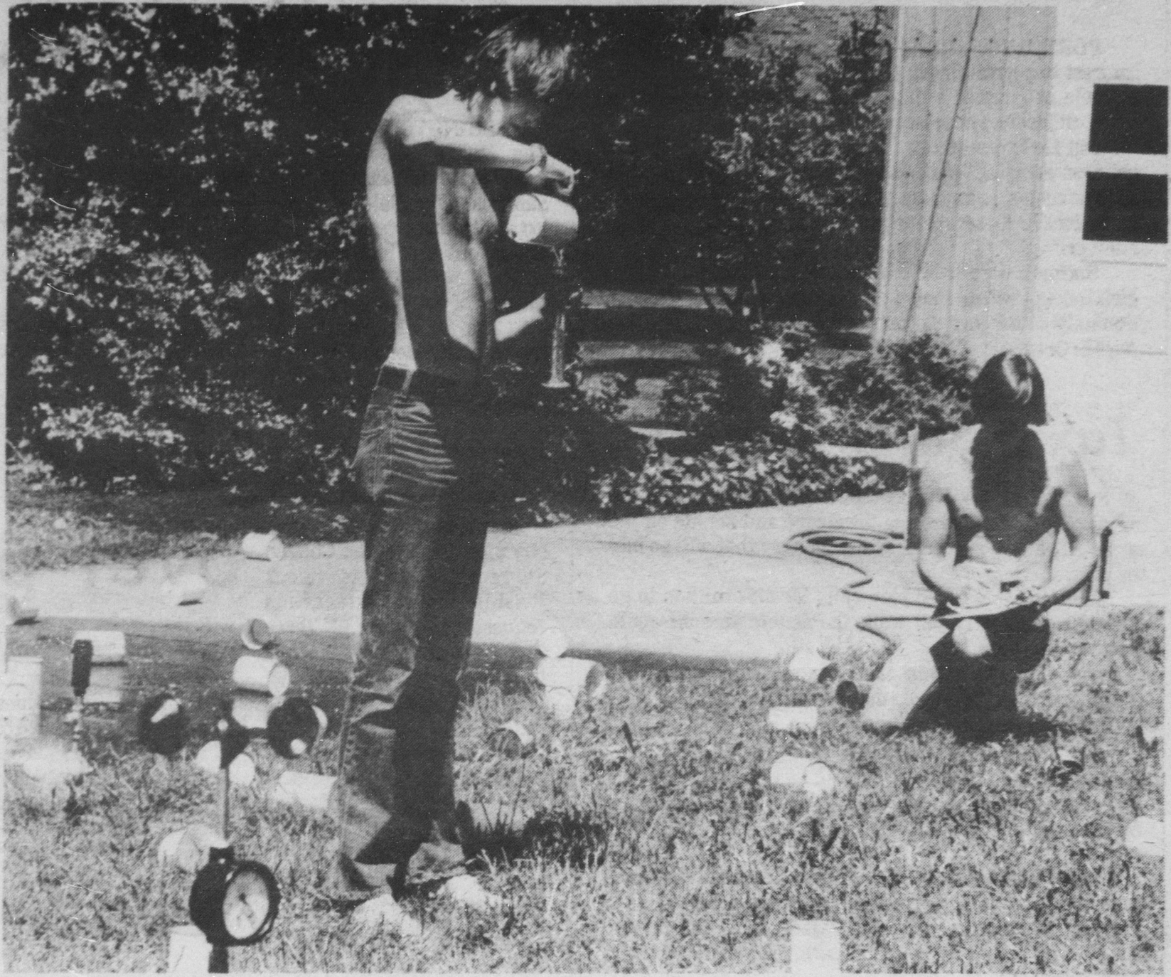
Steve Houghton, standing and Bill Traver both Juniors in Landscape Design, conduct a sprinkler uniformity test near the Farm Crops Building. The test is used to measure the flow of water using various sprinkler heads and to check water dispersal. (Photo by Tim Bernard)
