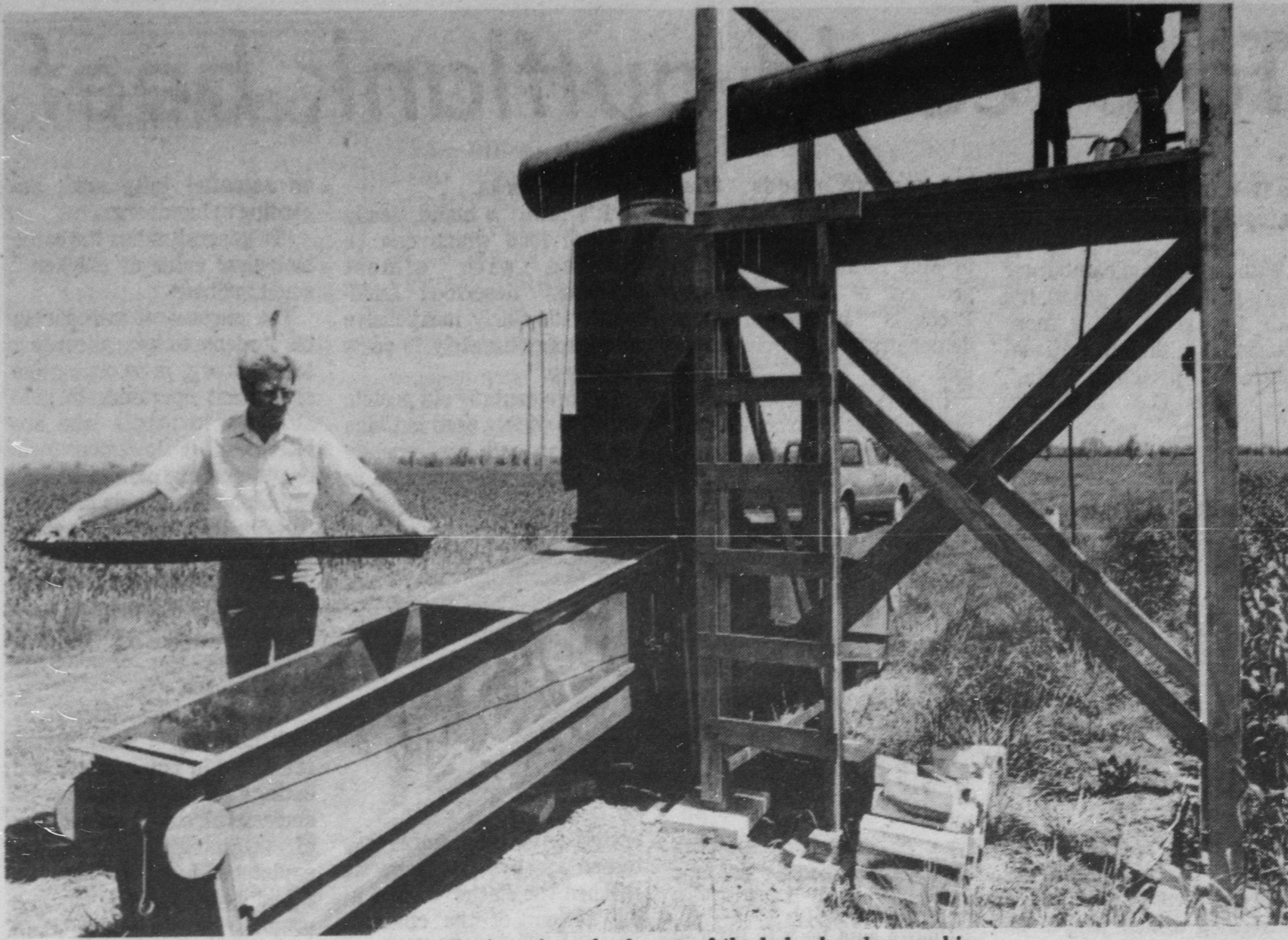
Glen Page, associate professor in Ag Engineering, checks one of the bale chambers on his own "straw bale burner" to be used as field and straw burning experimentation. (Photo by Ross Anker)
