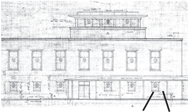
Dwg #1: Original Elevation c. 1948 showing original size of first-floor windows (single wide).
