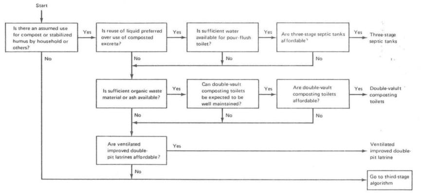
Figure 9-3 Third-stage Algorithm for Selection of Sanitation Technology
