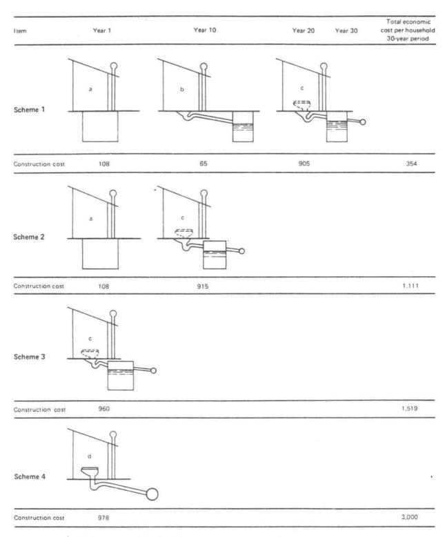
a, Ventilated improved pit latrine; b, pour-flush toilet with soakaway; c, pour-flush toilet with small-bore sewer (with optional bowl and seat); d, conventional sewerage.
