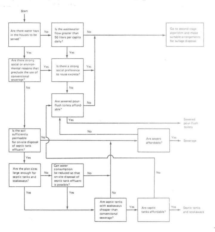
Figure 9-2 Second-stage Algorithm for Selection of Sanitation Technology ·
