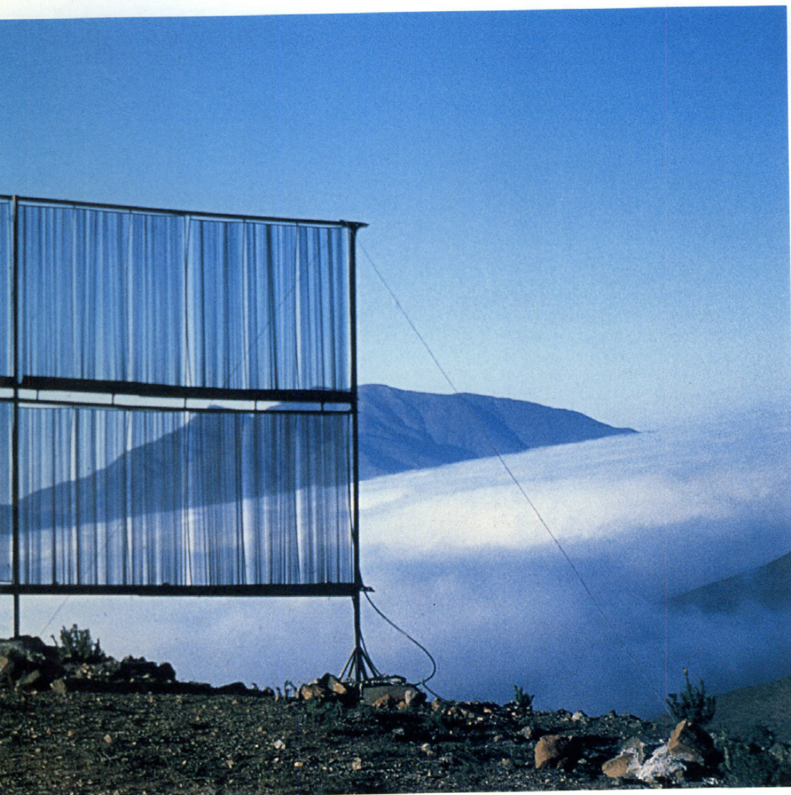
The strips in this screen serve to trap moisture from clouds and mist. The technique, developed in the Andes, is now also used in India and the Gulf region.
