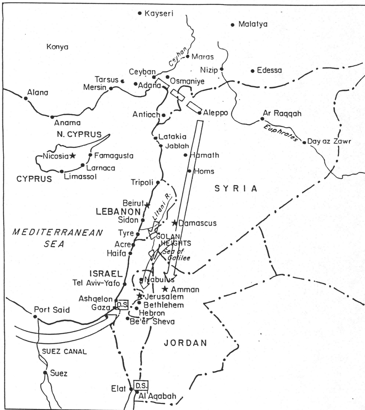
Figure 2 . Proposed alternative or complementary projects for bringing in additional water supplies to meet the long term needs of Jordan, Israel and the Palestinians which should be evaluated as part of a multi-billion dollar Water-for-Peace Plan. The following pipelines are proposed for evaluation: Nile River to Gaza Strip and the Negev ; Litani River in Lebanon to West Bank and Israel; Turkey to Syria, Jordan, and the West Bank. Major seawater desalination plants (DS) could be built on the Mediterranean coast between Israel and Gaza and on the Israel-Jordan border between Aqaba and Elat.
