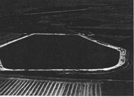
Yet another such reservoir was built a few years ago in Upper Galilee, near Moshav Dalton. Water from the Dalton Reservoir is used for irrigation in the local settlements. Last year the embankments forming the reservoir were raised in order to increase its capacity.
