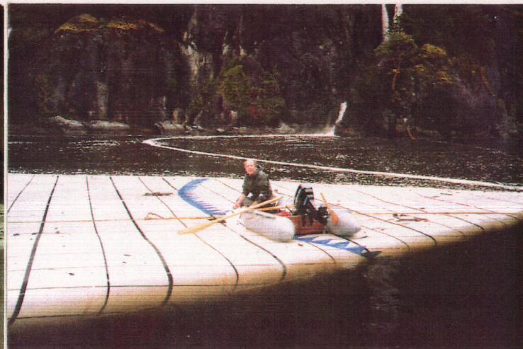
Prototype filling from waterfall. Tension supports weight of man and boat.
