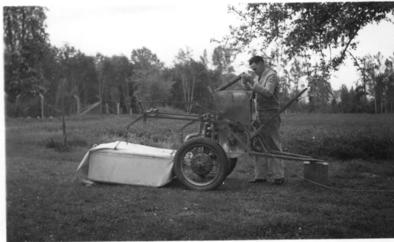
Fig. 15 - Side View of New Dusting Unit for Strawberries Note: - Both axel and hood are arranged to meet various widths of rows.
