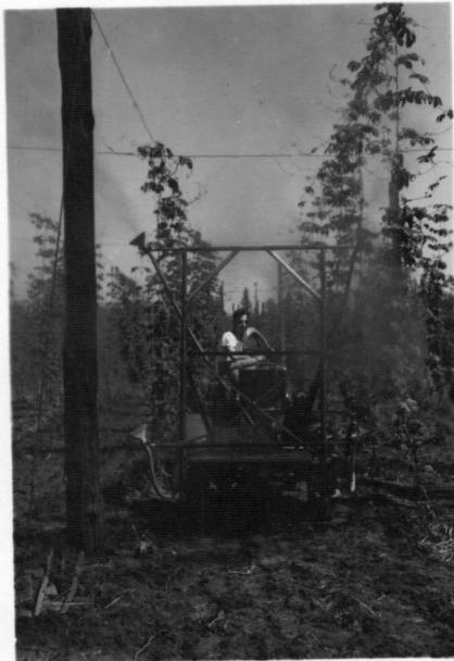
Fig. 7 - Rear View of Bean Dual Hop Duster. Note dust does not reach tops of hop vines.
