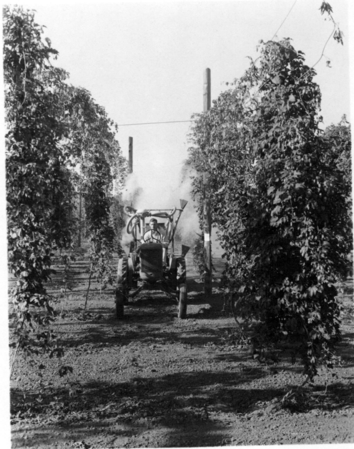
Fig. 3 - Improved Experimental Duster in Operation 1941 Station Field Day
