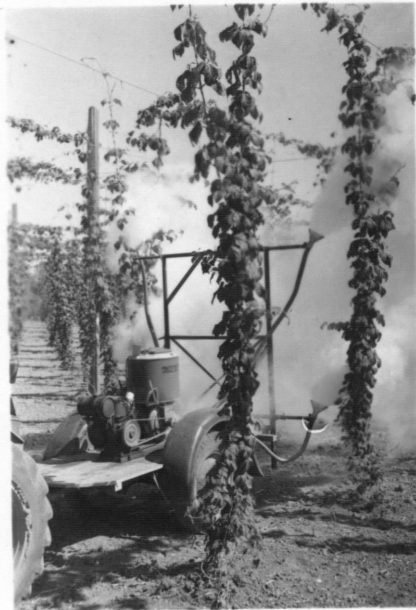
Fig. 6 - Bean Dual Hop Dusting Unit in Operation. Note dust does not reach tops of hop vines.
