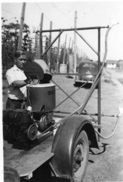
Fig. 5 - View of the Experimental Hop Duster Using a Bean Dual Unit. This unit did not have adequate capacity for hop dusting.
