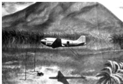
Illustration of snatch pickup, from 1944 US Army Air Forces manual.
