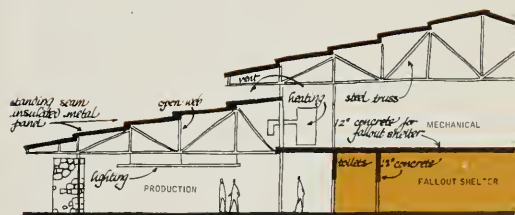
SECTION THROUGH FACTORY
