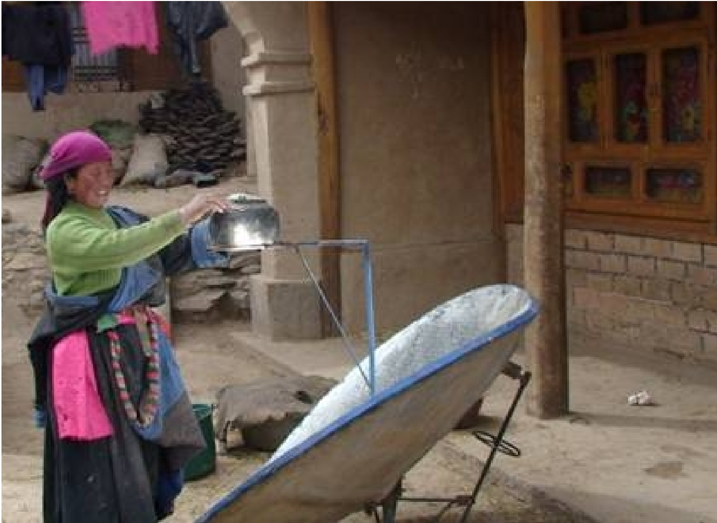
Lama Tsering (b. 1977) boils water on her new solar cooker. She used to burn collected yak dung for cooking. She still does but much less, especially on sunny days. She also spends much less time collecting yak dung.
