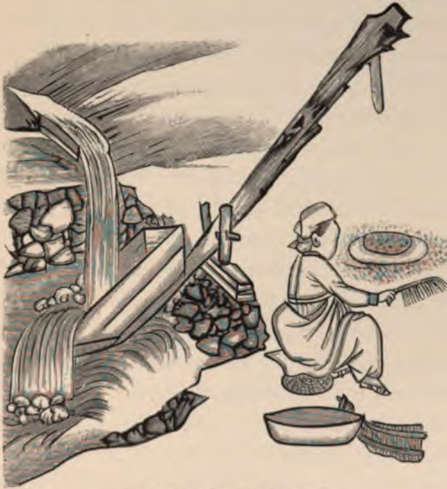
WATERMILL FOR HULLING RICE.
