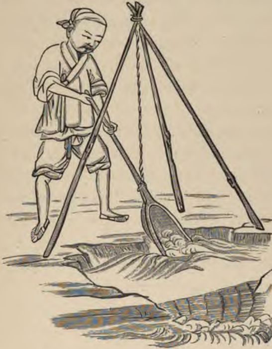
LIFTING WATER BY TRIPOD FRAME.
