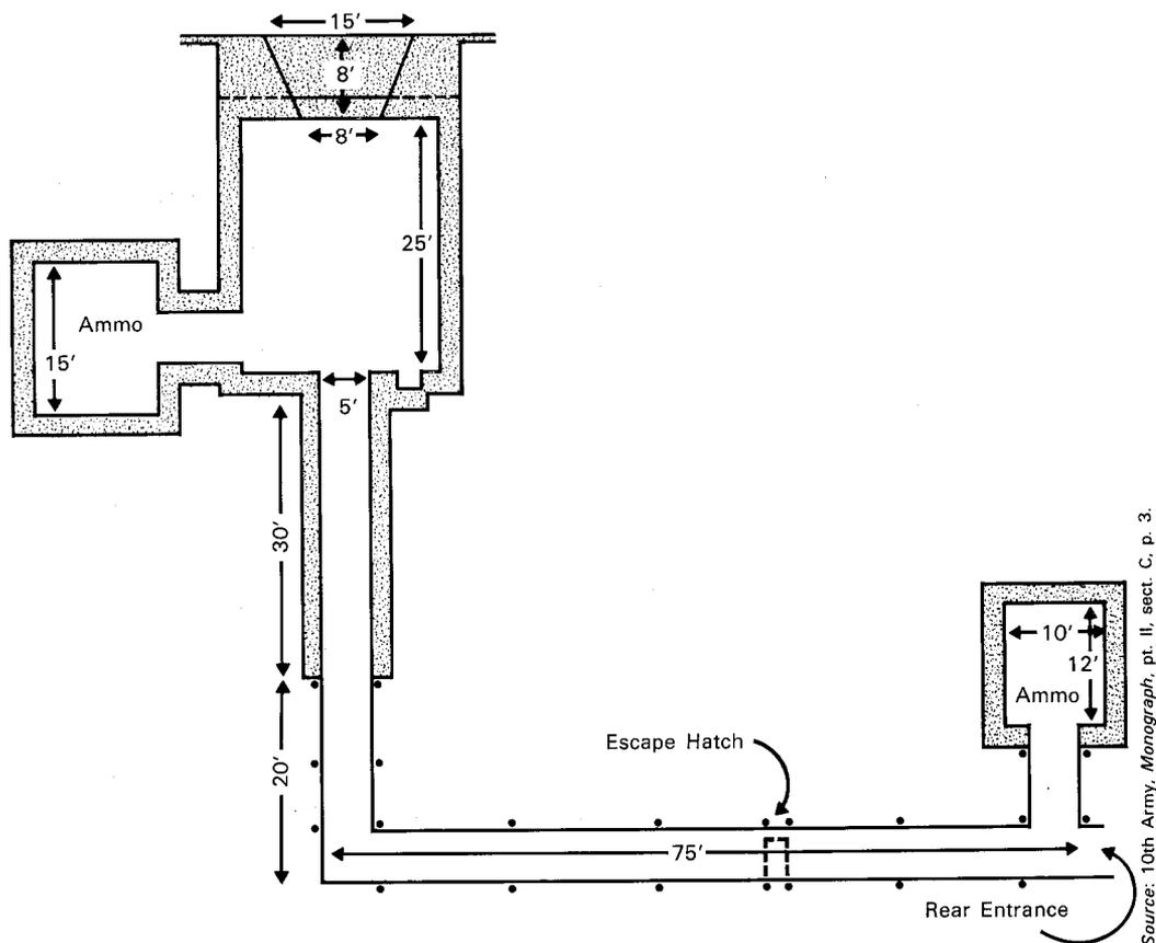
Figure 7. An IJN 150-mm naval gun position
