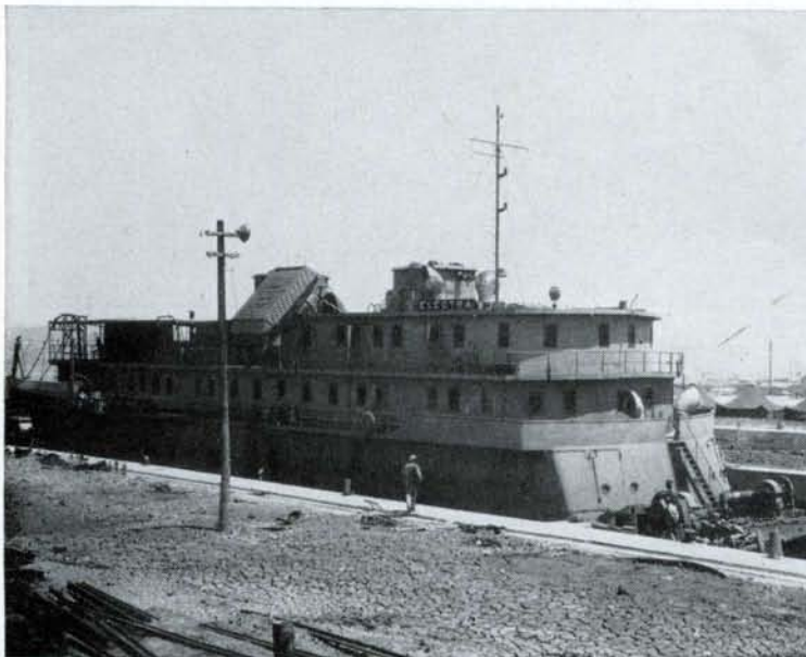
POWER OUTPUT CONTINUED. As Reds cut supply of power from North, U. S. barge-generators kept the South's industrial wheels turning.
