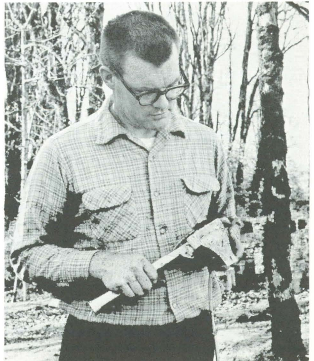
Mike Newton displays a device that he has developed for injecting herbicides into unwanted trees.
