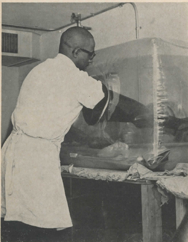
BELOW: Porter demonstrates how the arm-length, heavy-duty rubber gloves are used to minister to the small white animals.
