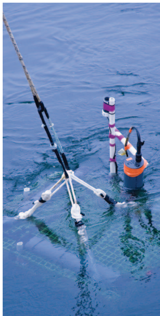
One of Schultz's monitoring devices, made mostly of plastic and held together with tape to avoid interference with magnetic and electrical measurements, is sent below to do its job. PHOTO BY DENNIS WOLVERTON
