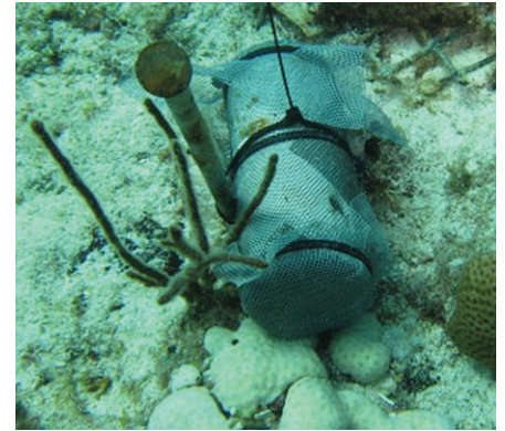
"Diffusers" such as this were used on coral reefs to slowly release nitrogen and phosphorus and raise the levels of those nutrients in nearby sea water. (Photo courtesy OSU)
