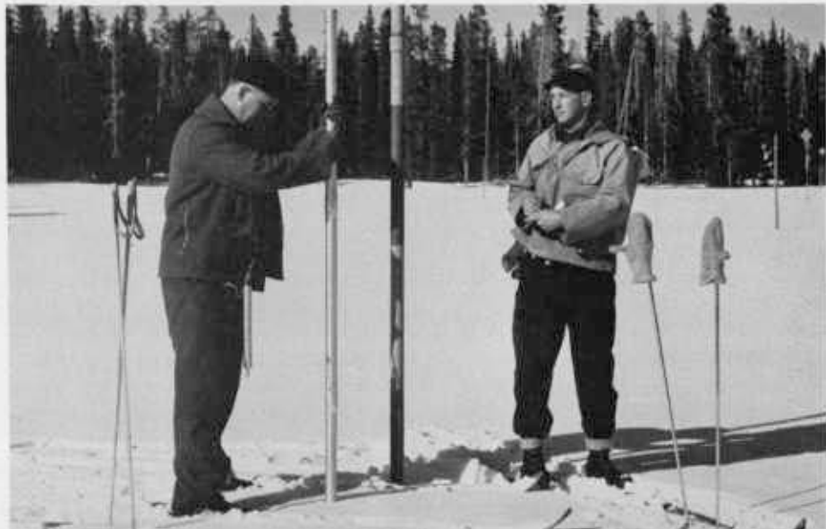
R. A. WORK (left) and A. E. Kenworthy sink a 1½-inch aluminum tube through the snow for sample. Pipe at right is snow course marker. Some 175 snow surveyors visit 126 courses to obtain samples.
