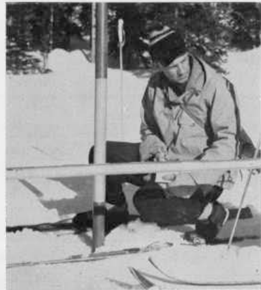
AMOUNT OF WATER in snow sample is weighed and about 10 samples each visit to snow course—once or
