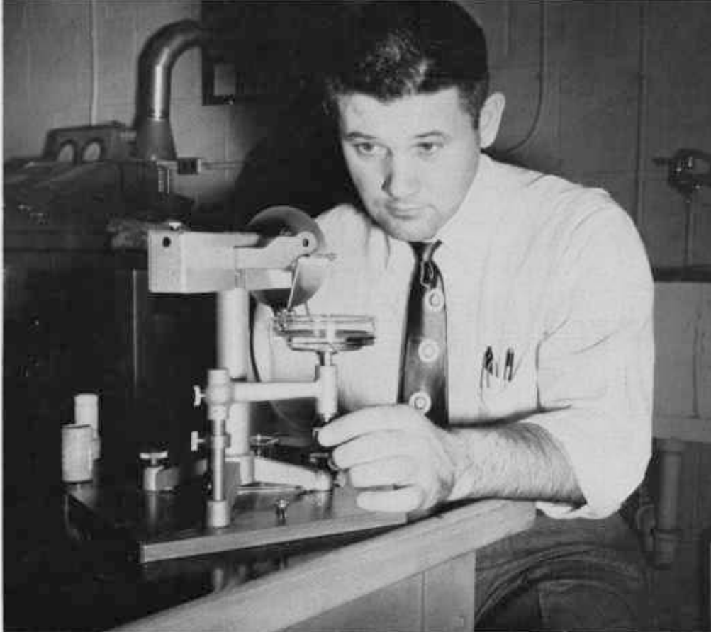
AGRICULTURAL CHEMIST Virgil Freed checks a reading on a tensiometer, an instrument he uses to measure a solution's surface tension. A low surface tension means better wettability, higher kill.
