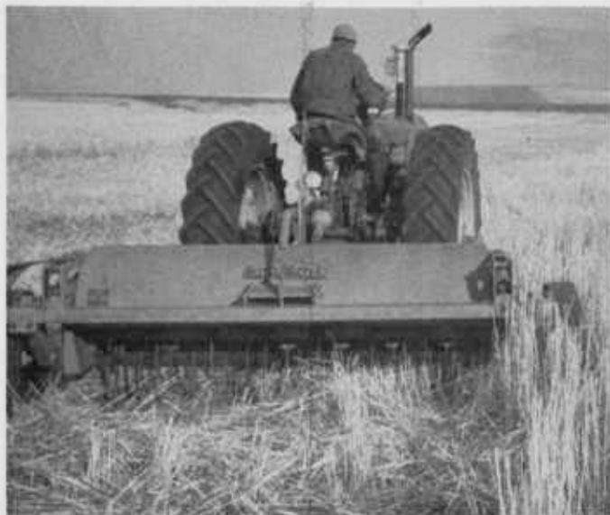
Stubble buster in action. Note how it breaks up straw. Next step is to work land with sweep plow. Skew treader not needed after buster.
