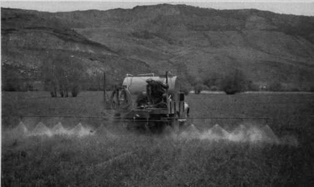
ABOVE, adjust pressure to 20 to 40 pounds per square inch. This is usually low enough so nozzles operate properly. BELOW, use nozzles that deliver a large-sized droplet, or about 1 quart per minute.
