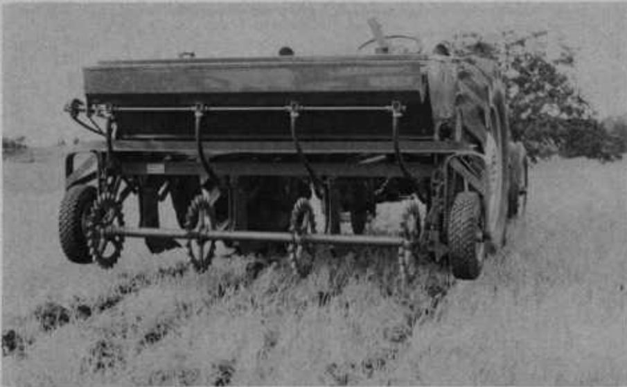
OVERALL view of the pasture renovator, or duck-foot plow, recommended for use in establishing sub-clover. This type of plow could probably be built by most farmers who have complete farm shops.
