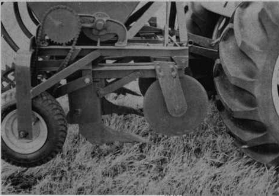
CLOSE-UP of the duck-foot plow. Main features are heavy shank, fertilizer applicator, and a seeding attachment. The shank must be strong enough to open a shallow furrow in hard, dry, soils.
