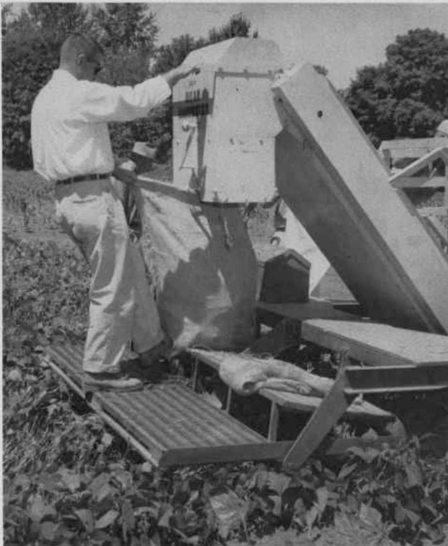
BEANS conveyed to rear of machine were collected in sacks during OSC trial demonstration. In commercial harvesting operations, beans drop into half-ton capacity pallet boxes mounted on rear platform.
