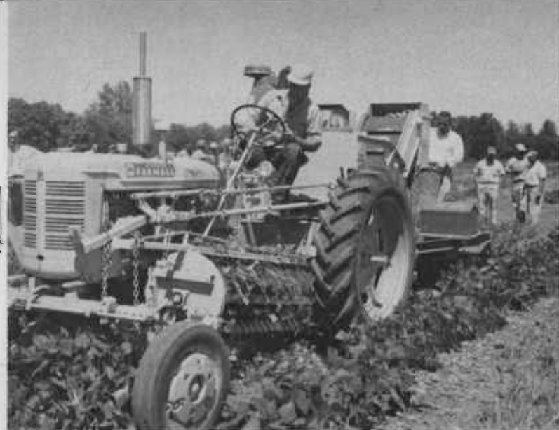
MECHANICAL bush bean harvester covers 3½ to 5 acres a day, travels about three-fourths mile an hour, picks from 15 to 20 tons of beans a day.
