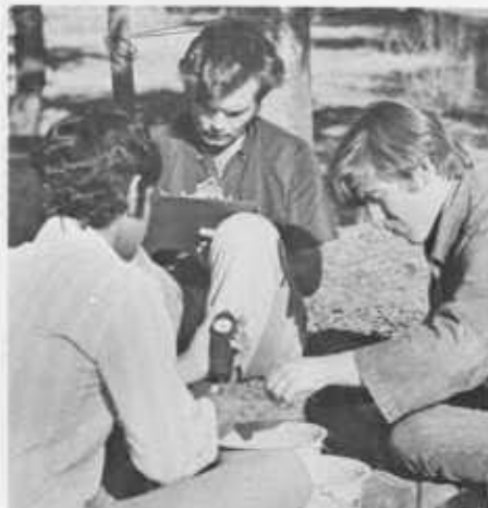
After setting accelerometers on the tree trunks (above) researchers used electronic equipment to monitor the tree movement (left). Force required to pull cherries from stems also was recorded (below).
