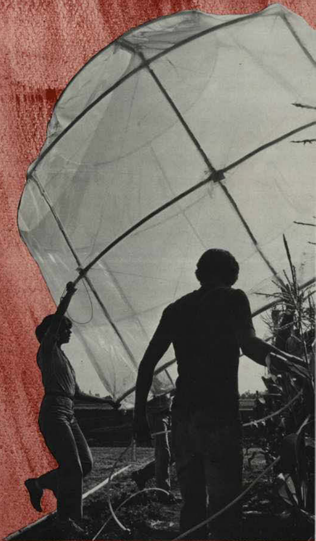
Left: Crop scientist Cynthia Cohen. Above: Mobile plastic bubbles are used at OSU's Schmidt Farm to cover field crops (corn here) during simulated rain events. Right: Workers lift a bubble over test plots.
