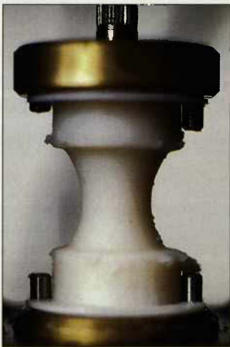
Quality is determined by texture and cohesiveness. This cooked surimi is undergoing a torsion test.
