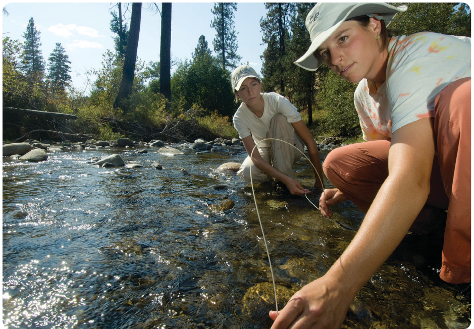
OSU graduate students Julie Gabrielli (foreground) and Aida Arik place a fiber optic cable into Big Boulder Creek to measure water temperature all along this tributary of the Middle Fork of the John Day River.
