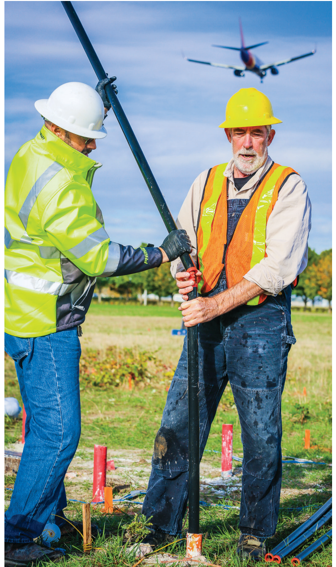
OSU's Armin Stuedlein, left, worked with blasting expert Jerry Wallace and OSU student researchers on a project near Portland International Airport in which underground detonations helped reveal what might happen to the airport's runways in a major earthquake.
