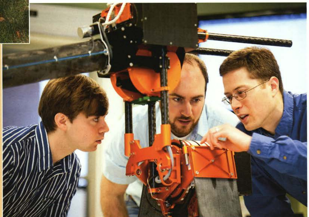
Right: From left, students Christian Hubicki, Jesse Grimes and Assistant Professor Jonathan Hurst discuss details of the wire routing on the prototype running robot ATRIAS.
