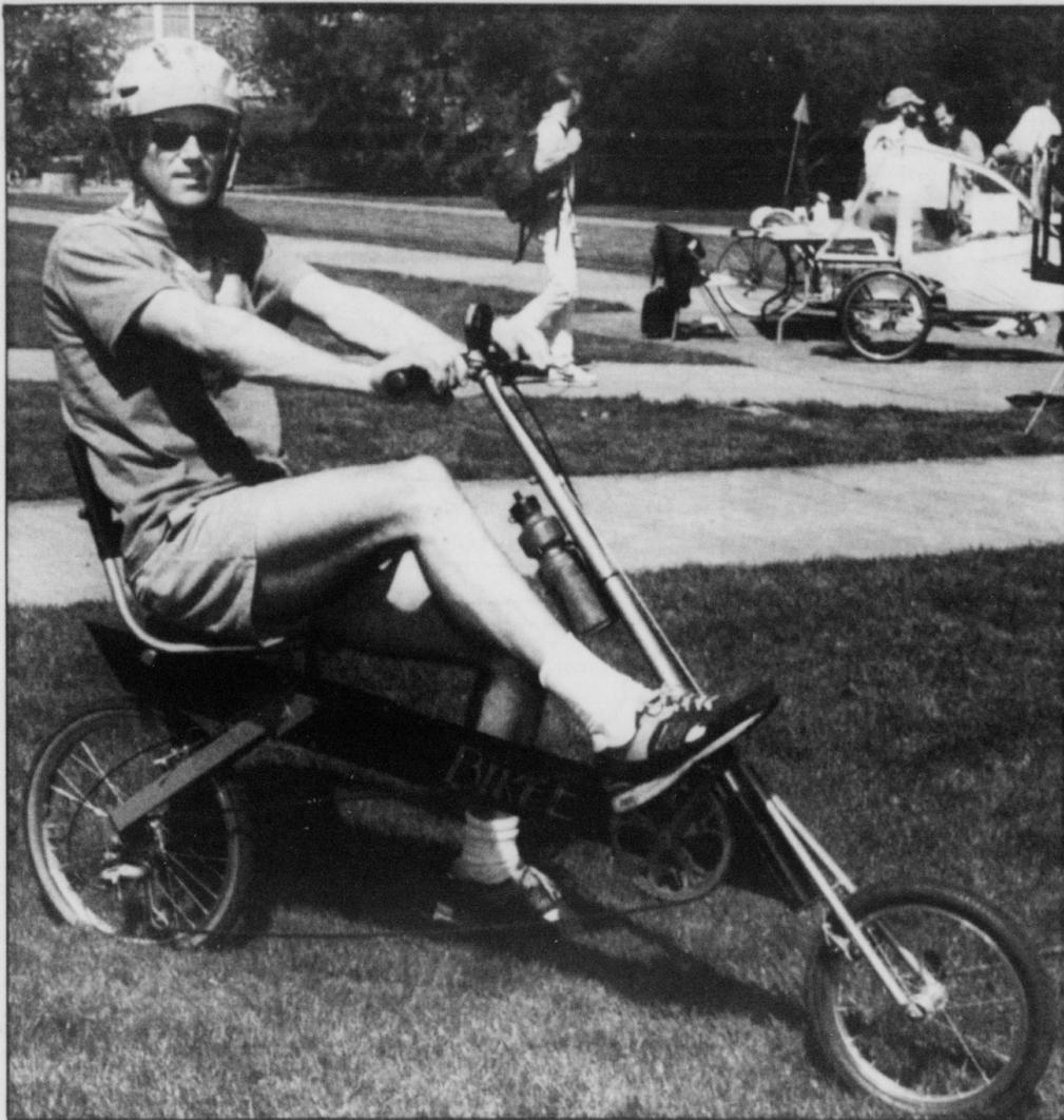
Jim Boeder, marketing director of BikeE Corp., demonstrates a new style of recumbent bicycle. A recumbent bicycle is one in which the rider sits upright or in a reclined position, and is closer to the ground than on a conventional bicycle. Recumbent bicycles are becoming more popular than the conventional bicycle because of its better weight distribution and because the rider is in a more upright position.
