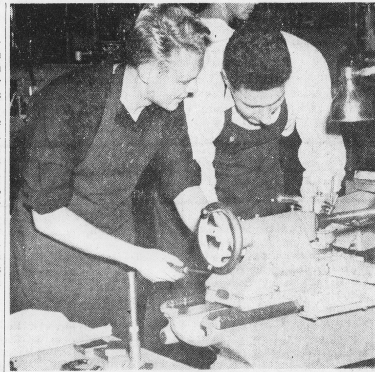
TWO OSC STUDENTS set up a screw-cutting lathe for a taper-turning job in the industrial arts lab. Photo by Wally Johnson.
