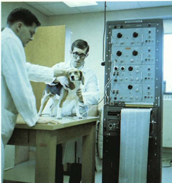
The dog's blood pressure, heart rate and respiratory activity are measured on a polygraph.
