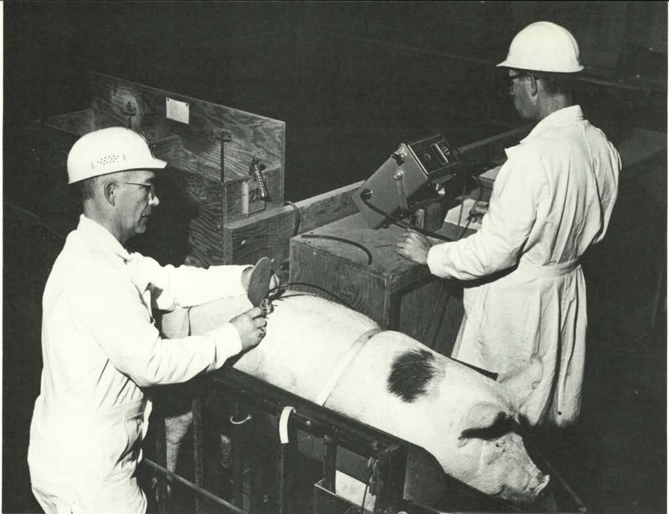
An electronic device is used to measure the thickness of back fat on breeding animals.
